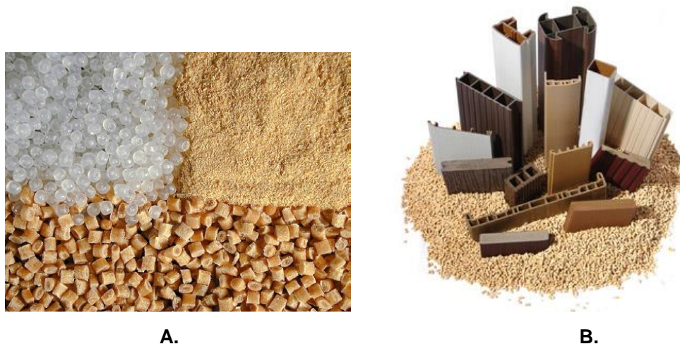
Figure 1 A: The granules from the wood and thermoplastic; B: The WPC products
