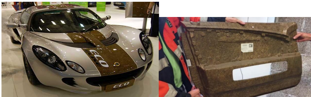
Figure 7 Hemp fibre reinforced polymer composite
