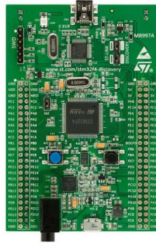
Figure 4 STM32F407VG Development Board
