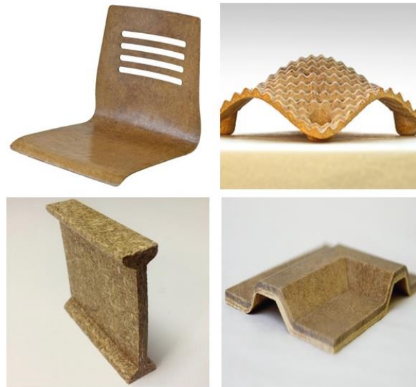
Figure 2 Examples of biocomposites produced using sugarcane particles NaturoMer® (Anonymous, 2021)
