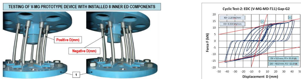
Figure 2 Cyclic testing of V-MG-ED devices (left) and Performance of EDC with simulated gap-G2 (right)
