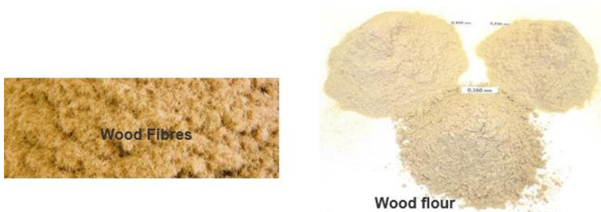
Figure 2 Examples of wood fibres and wood flour used in the WPC production
