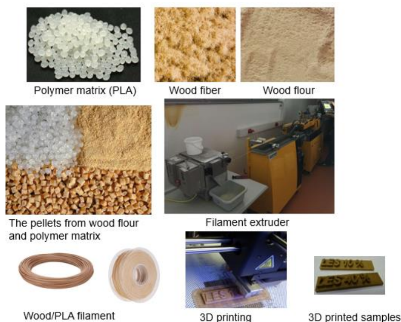
Figure 2 Raw materials, production of filaments and 3D printing of the filaments
