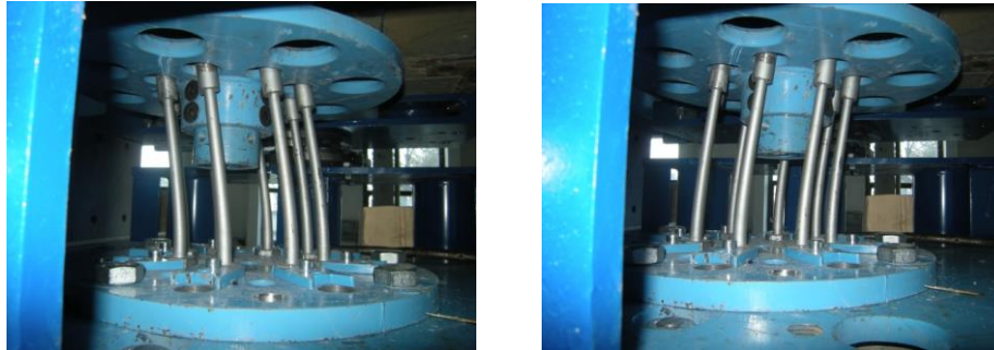
Figure 3.1 Laboratory tested model prototypes of new seismic energy dissipation devices (EDD) of vertical V-Class under simulated earthquake-like reversed cyclic loads: Type 1: EDD-V-T1 and Type 2: EDD-V-T2
