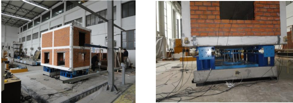
Figure 4.1 View of constructed large-scale building model tested on seismic shaking table (a) and detail of seismic isolation and energy dissipation devices (b) of the proposed seismic protection system for buildings
