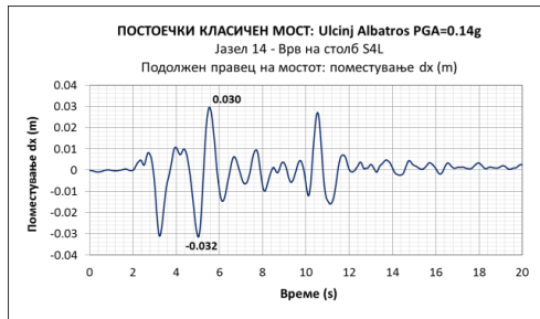
Fig. 4.1. Time history response of the displacement dx (m) at the top of pier S4L in longitudinal direction of the bridge
