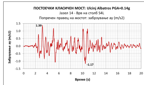
Fig. 4.2. Time history response of the acceleration ay ( m/sec^2 ) at the top of pier S4L in transversal direction of the bridge
