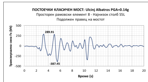
Fig. 4.8. Time history response of shear force F_X (kN) at the bottom of pier S5L: Longitudinal direction
