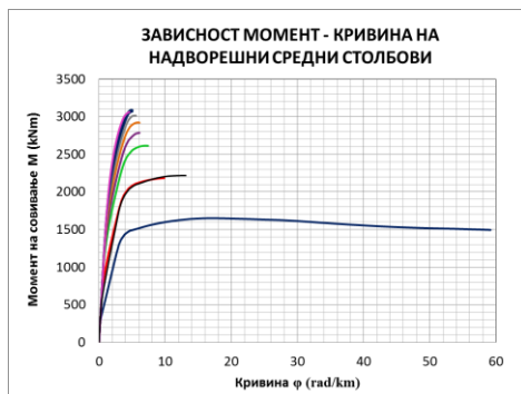
Fig. 3.3. Moment-curvature (M- \phi ) relationships for the piers S2 and S5 for different levels of axial (N) forces
