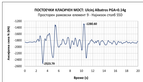
Fig. 4.7. Time history response of axial force N (kN) at the bottom of pier S5D: Axial direction
